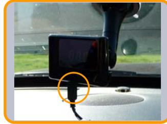
An immediate audible “Beep” sound will indicate the display unit is on. In 2 to 3 minutes, the display unit will show the tire pressures in yellow, along with four blue tire position lights.
