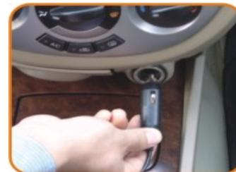
3.1.2 Plug the power cord into the display unit and plug the adapter into auxiliary power supply.
